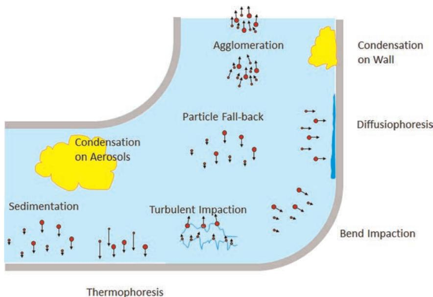
Fig. 5. Main phenomena in the fission product transport module in the reactor circuit of ATHLET-CD/AC<sup>2</sup>
