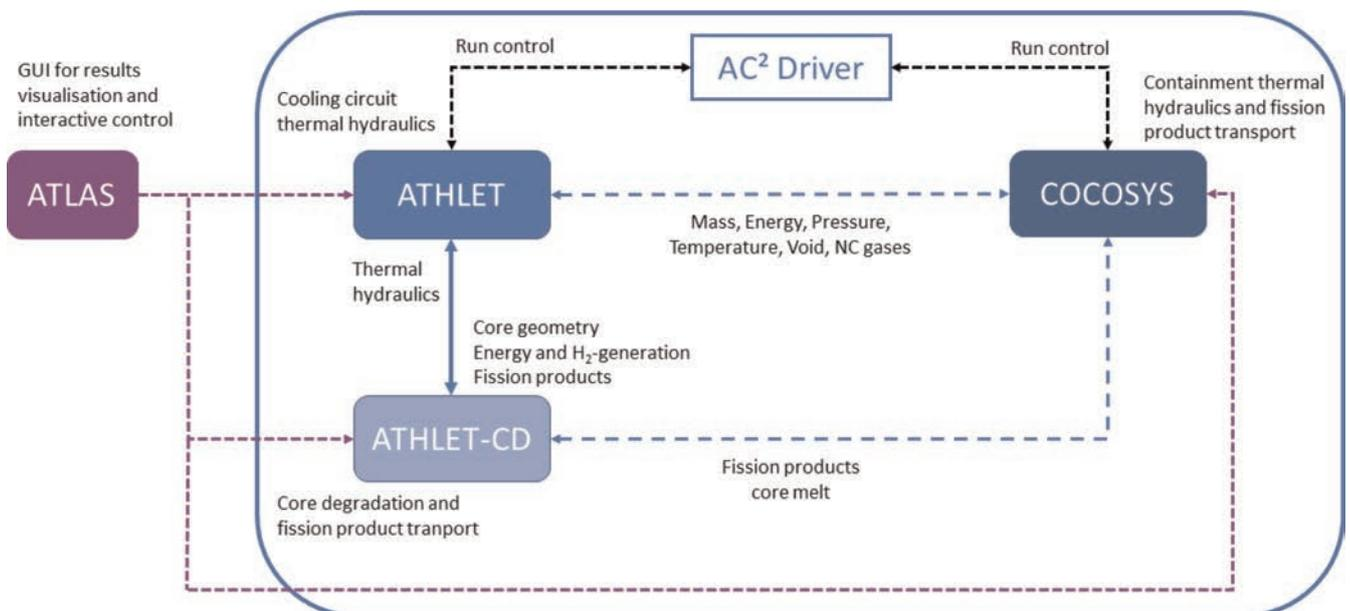
Fig. 1. Link between main modules of AC<sup>2</sup> (picture taken from [2])
