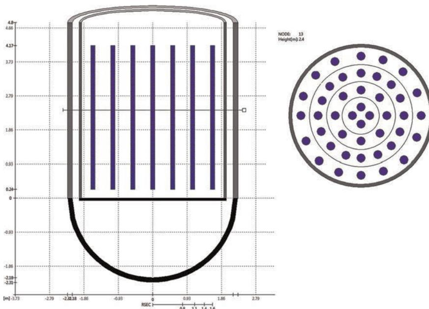
Fig. 4. Side and top view of the core nodalization in ATHLET-CD/AC<sup>2</sup> (from [4])
