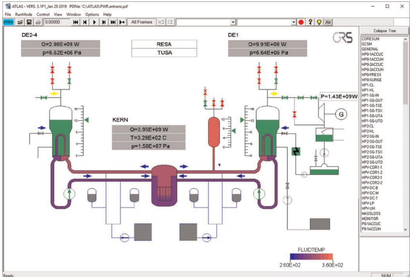
Fig. 8. ATLAS user interface for postprocessing and interactive control of AC<sup>2</sup> simulations (GRS)
