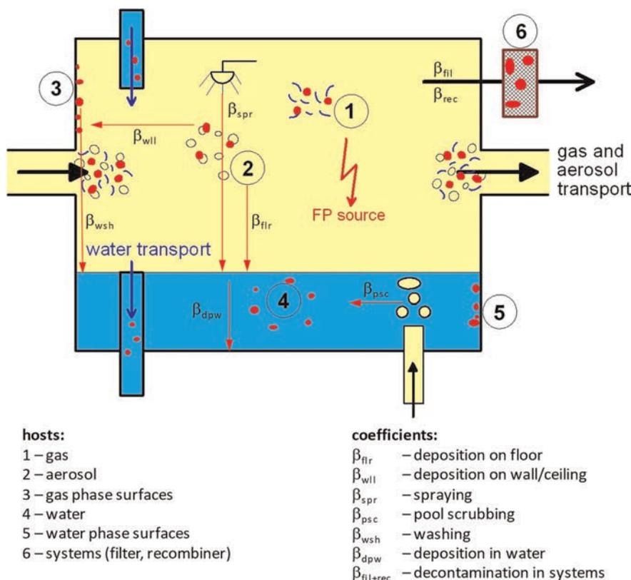
Fig. 7. Main aerosol and fission product phenomena simulated in COCOSYS/AC<sup>2</sup> (from [8])
